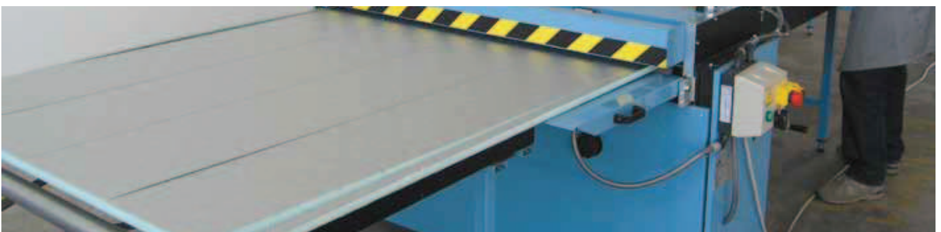
[Focus on cut panel exiting the automatic straight cut machine]
